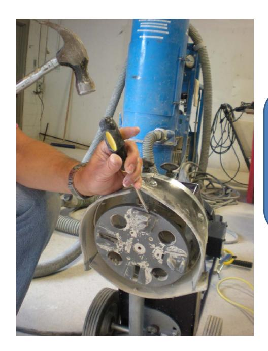
Note using the TEQLOK quick change tooling is to use something like a flat screwdriver to gently tap the lock free. Do not hit the diamond segment with a hammer because it can damage it.
